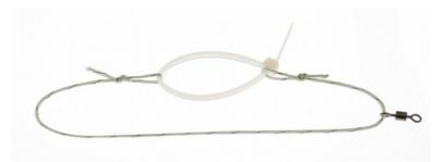
Two overhand-loop knots are used at each end of the line to provide loops for the zip-tie to go in-between. The finished line length, from loop-to-loop, should be 20 cm. A swivel is placed between these two loops to attach the load line to.
