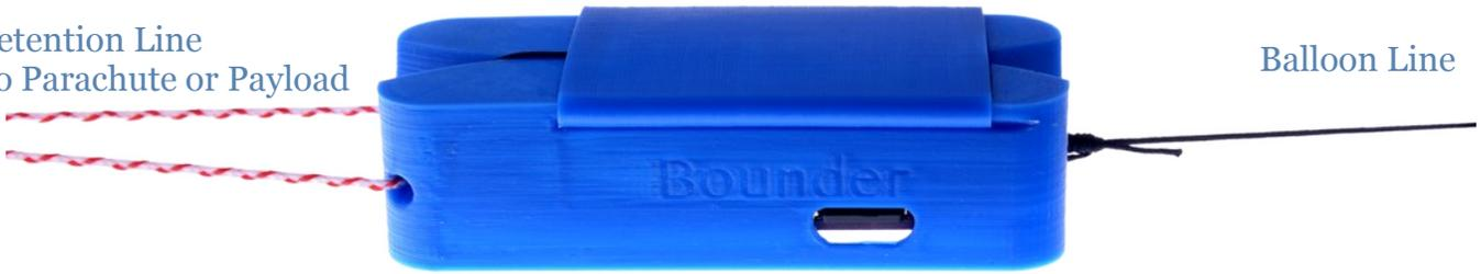
The retention line (pictured as red/white above) is tied through the provided hole to ensure the *Bounder* isn't lost after burn-wire activation.
