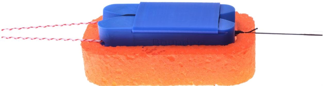
The *Bounder* ships with a radiative insulation device. This device (the blue cover) slides over the batteries and helps ensure that they stay warm at high altitudes. Please ensure the batteries are not touching the radiative shield after installation, as shown in the photo below.
